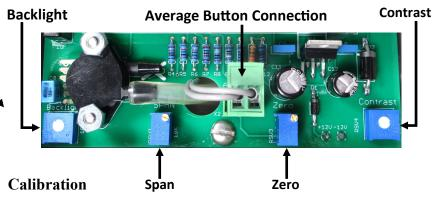
Unit is factory calibrated. If calibration is needed: Calibrate the gauge using the zero and span pots. (See picture above.) With no vacuum applied the Screen should display 0.00" Turn zero pot clockwise to increase, counterclockwise to decrease. Apply 12" or higher of vacuum, use a calibrated meter to verify the vacuum level. Adjust span to match known level, clockwise to increase, counterclockwise to decrease. Repeat procedure until display is accurate at 0.00" and high vacuum.
